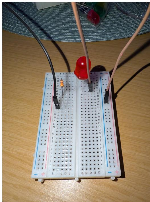
6. Connect a male to female cable from the top of the blue railing to any pin labelled GND on the pico
