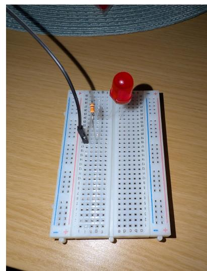
5. Connect a male to male cable from the short leg of the LED to the negative (blue) rail on the side
