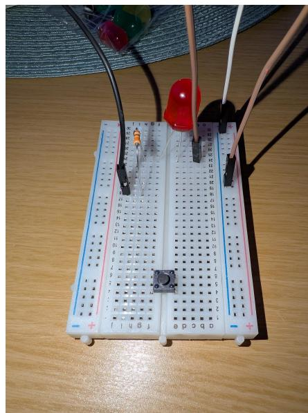
8. Connect a male to female cable from the button leg on the left hand side of the breadboard to pin GP18 on the pico
