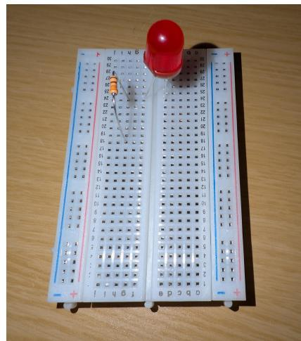
4. Connect a male to female cable to the same row as the resistor. Connect the female end to the pico to the pin labelled GP20
